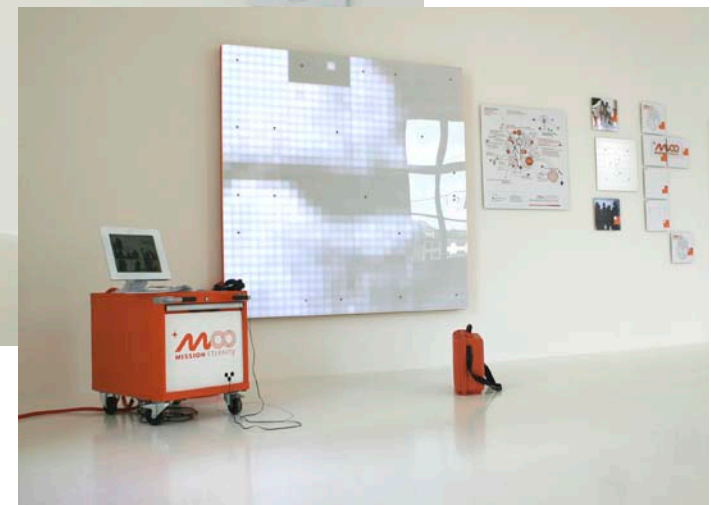
Material: M∞ DISPLAY (2 m x 2 m) outfitted with 2'048 high power LED pixels and LISTA server wagon including voice control, LCD screen.
